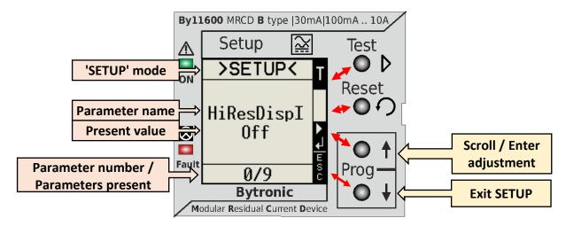
The right part of the display is related to the function of the adjacent keys, and each time in the 4 areas there are indications on the function of the relative key.
