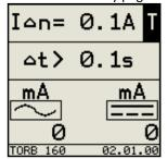
Remember also that with TORB160 and 210 it is possible to select the 0.1A range but there could be a greater measurement error of the DC component, which in any case does not exceed +/- 10%.
