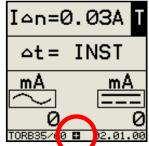
When the instrument is set up for protection against indirect contact ( $I_{\Delta n}$  = 0.03 A) no delay can be set. Delay  $\Delta t$  is adjustable only if  $I_{\Delta n} > 0.03$  A
