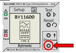
The 'DOWN' key has multiple functions, depending on the context of operation of the instrument.
