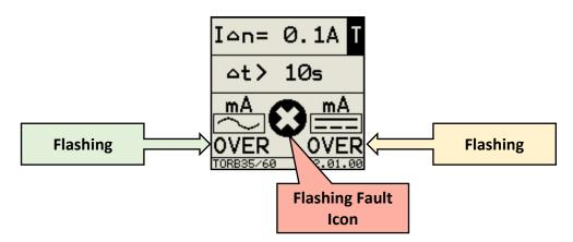
At the end, after  $\Delta t$  the Fault test trip will take place and, releasing the Test button, the negative R will appear in correspondence with the Reset button. See paragraph 'Reset'.
