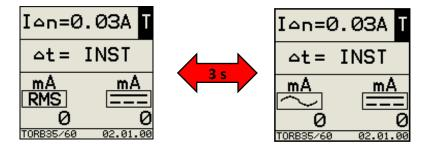
The 'INFO' bar contains the type of detection device associated on the left and firmware version information on the right. **CAUTION**: this is the setting for protection against indirect and additional contact against direct contact ( $I_{\Delta n} = 0.03A$ ). This setting is NOT POSSIBLE if TORB 110, TORB 160 or TORB 210 are used (the instrument does not admit 0.03 A selection). In case of use with TORB 110, TORB 160 or TORB 210 the first factory page will be the following (ex. TORB 160):
